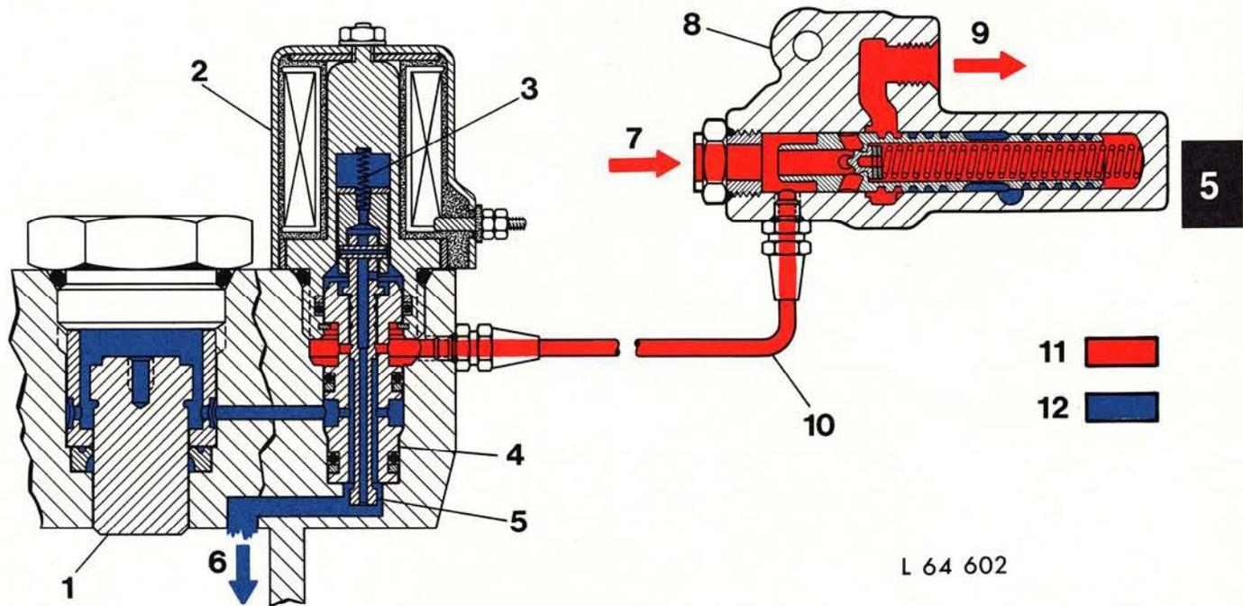
Fig. 7 — Oil Flow with MFWD Disengaged
