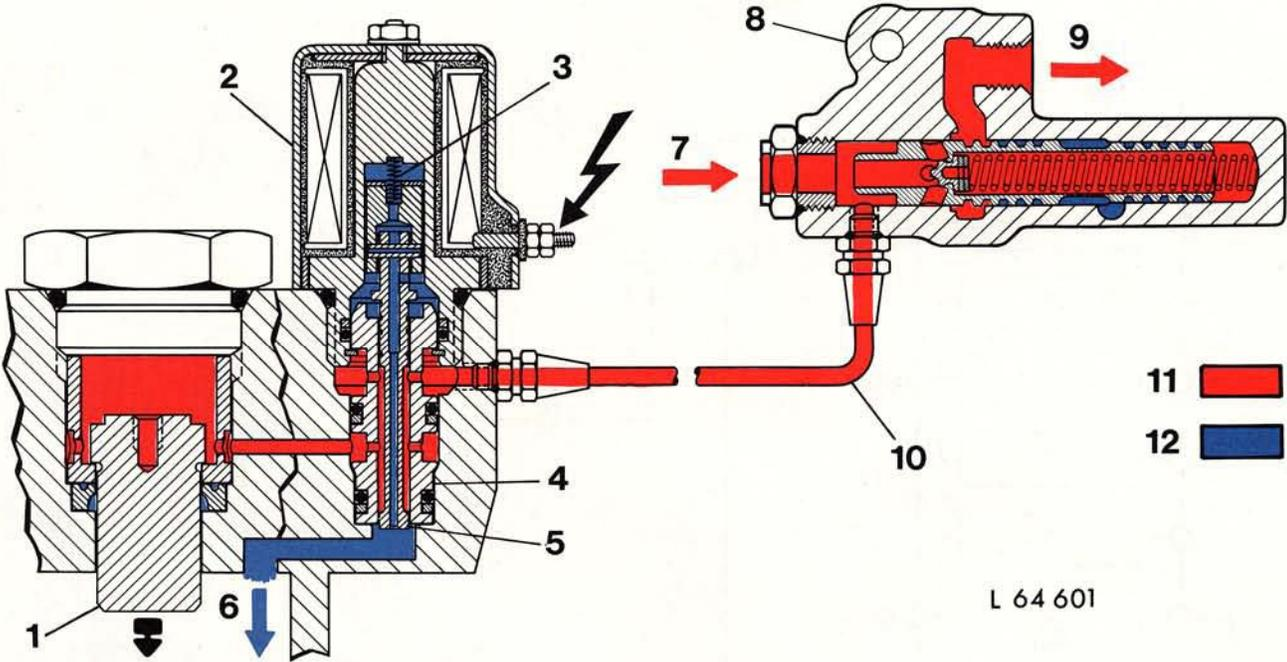
Fig. 6 — Oil Flow to the Clutch Piston with MFWD Engaged
