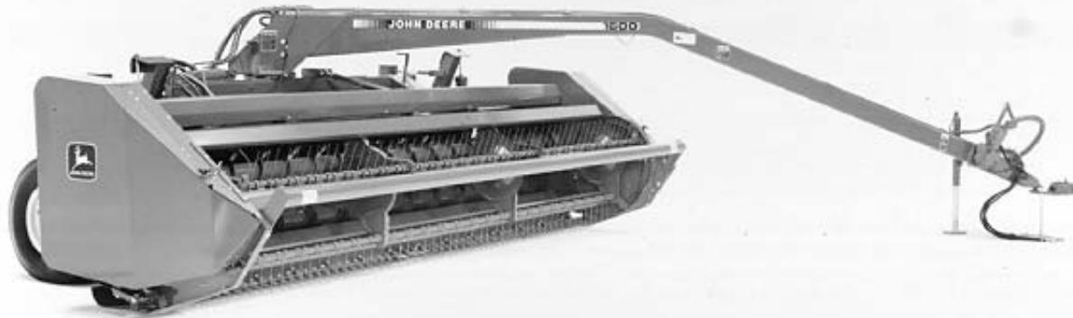
The John Deere 1600 Mower-Conditioner is a mid-pivot design which allows cutting back-and-forth or around the field. Machine raise and swing are controlled by tractor hydraulics, and a PTO hydrostatic pump drives the power train. The platform
