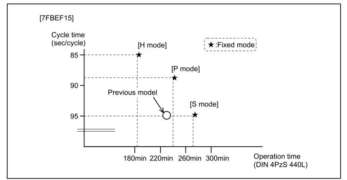
Especially, the loaded traveling and material handling performances in the H mode have been improved over 30%. As a result, our 30-m operation cycle time has been shortened by about 10% or more.
