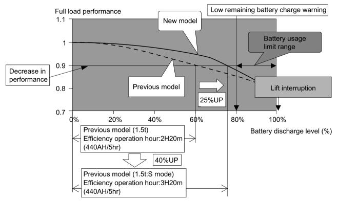
However, note that efficient operation becomes hard when the battery level indicated by the battery charge indicator becomes one bar (battery discharge to about 90%).
