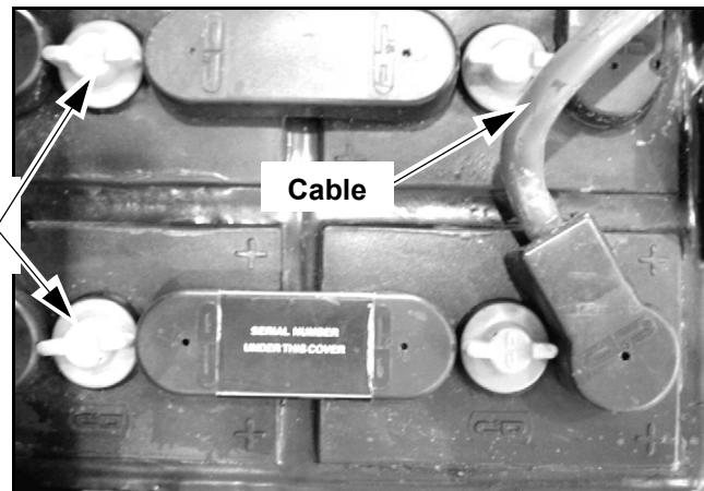
Keep filler plugs firmly in place at all times except when the electrolyte level is checked, when water is added to the cells or when the specific gravity is checked.
