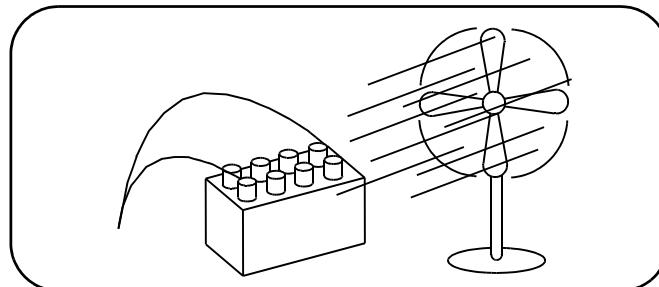
Press the red OFF (O) key on the keypad before disconnecting the battery from the truck at the battery connector. Do **NOT** break live circuits at the battery terminals. A spark often occurs at the point where a live circuit is broken.
