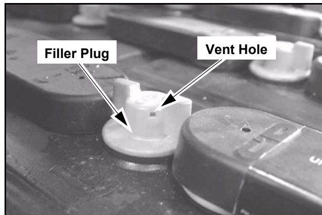
Do **NOT** allow cleaning solution, dirt, or any foreign matter to enter the cell.
