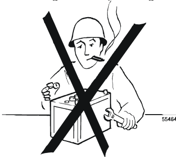
Figure 2 Do not smoke near batteries!
