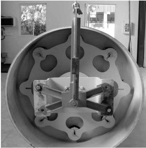
Figure 2 Tool assembled to the drum drive motor mounting bracket
