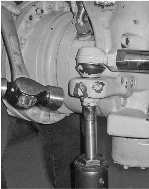
Figure 2 Tapping the spindle to release the ball joint
