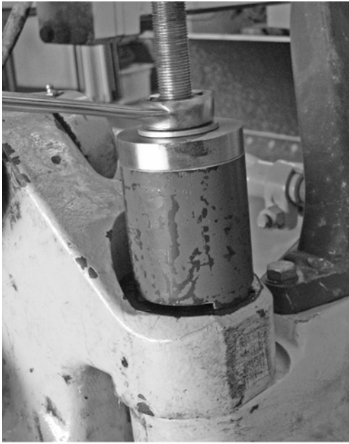
Figure 4 Removing the king pin from the spindle using a puller
