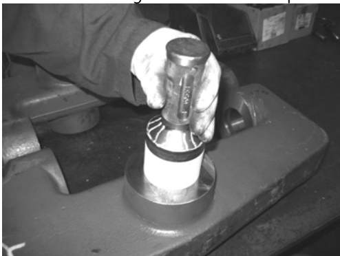
Figure 10 Driving the bushing into the axle pivot bore
