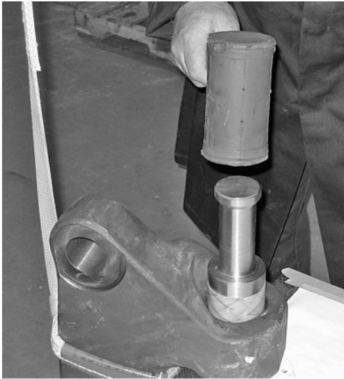
Figure 8 Installing new bushings into the knuckle
