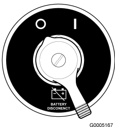
Figure 19 Battery isolation switch
