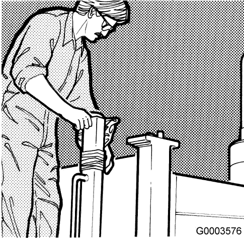
Figure 14 Removing cab plastic protective covering
