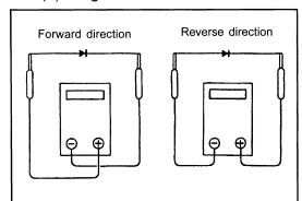
Measurement result example Tester range:  $M\Omega$  range
