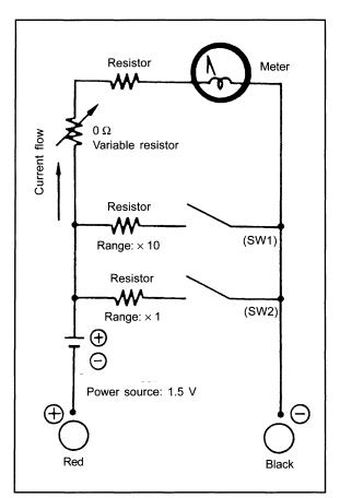
Always use the range described in the repair manual for measurement.
