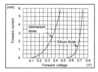
The resistance values of the same semiconductor measured with two types of circuit testers having different power supply voltages are different.
