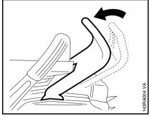
Disengage the chain brake by pulling the hand guard towards the front handle.
