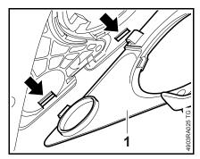
• Engage the cover (1) in the slots (arrows) first and then swing it into position.
