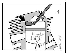
• The locking strip (1) 0000 893 5903 must butt against the cylinder wall (arrow) as shown.
