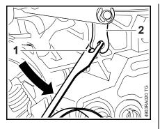
• Turn the brake band (1) to one side and disconnect it from the brake lever (2).
