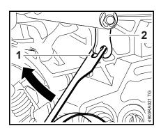
Hold the brake band (1) sideways, attach it to the brake lever (2) and then swing it in the direction of its seat.
