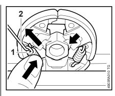
Attach the springs (1) on the side with the raised hexagon (arrow).
