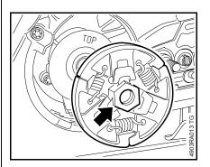
• Position the clutch on the crankshaft stub so that the raised hexagon (arrow) faces outwards.
