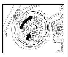
• Apply wrench to hexagon (arrow) and unscrew the clutch (1).
