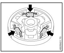
Check the clutch – all springs (arrows) must be properly attached.
