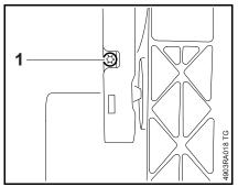
• Fit the screw (1) on the underside of the machine and tighten it down firmly.
