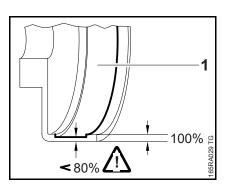
Inspect the clutch drum (1) for signs of wear.
