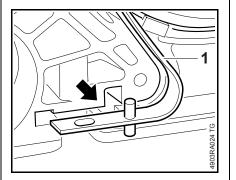
• Push the brake band (1) into its seat (arrow) as far as stop.
