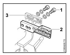
Servicing and repairs are made considerably easier if the machine is mounted to assembly stand (3) 5910 890 3100. To do this, secure the mounting plate (2) 5910 850 1650 to the assembly stand with two screws (1) and washers.
