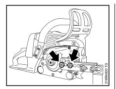
Engage the bar mounting studs in the outer bores in the mounting plate and secure the machine in position with the nuts (arrows).
