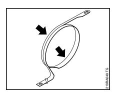
Install a new brake band if there are noticeable signs of wear (large areas on inside diameter and/or parts of outside diameter – arrows) and its remaining thickness is less than 0.6 mm.
