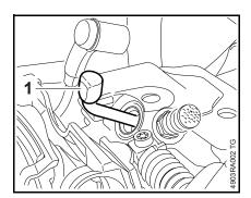
Push the locking strip (1) 0000 893 5903 into the spark plug hole, wide end first, so that "OBEN-TOP" faces up.
