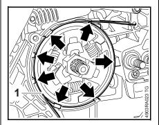
• Push the brake band (1) over the guide lugs (arrows) and into its seat.
