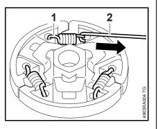
• Use hook (2) 5910 890 2800 to remove the clutch springs (1).
