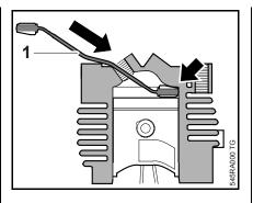
Push the locking strip (1) 0000 893 5904 into the spark plug hole until it butts against the cylinder wall (arrow) as shown.
