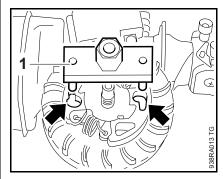
Position the wrench (1) 4130 890 3600 on the crankshaft stub so that its pins engage the recesses (arrows).
