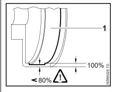
Inspect the clutch drum (1) for signs of wear.
