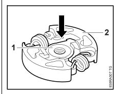
• Push the carrier (1) out of the clutch shoes (2).
