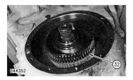
1. Install clutch hub (32) to the transmission.
