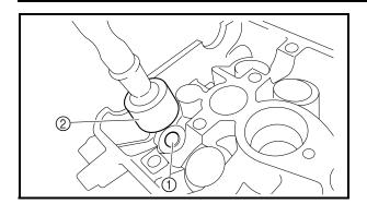
Install the new valve pad ① and the valve lifter
