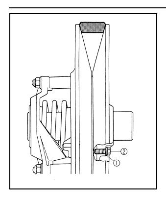
2. Adjust the position of the V-belt by removing or adding a spacer ① on each adjusting bolt ②.
