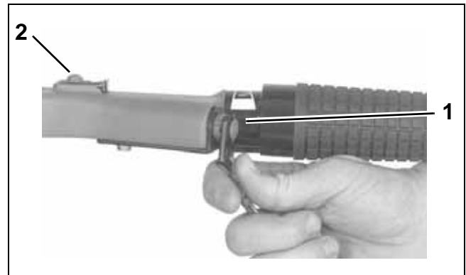
1. Emergency stop switch 2. Extra clip
