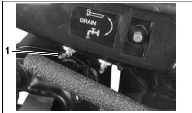
1. Drain valves in drain position
