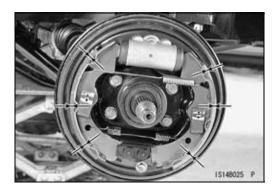
Brake Wheel Cylinder Assembly Replacement (Front Brake Panel)
