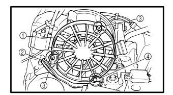
• Install the driven pulley outer sheave ③.
