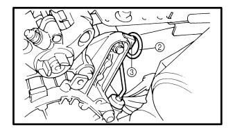
Reinsert the dipstick and fit the loop ② of the dipstick handle onto the projection ③ of the gear case.
