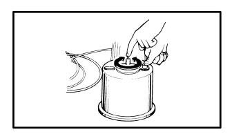
If necessary, clean the spark plugs with a spark plug cleaner.
