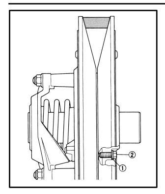
2. Adjust the position of the V-belt by removing or adding a spacer ① on each adjusting bolt ②.
