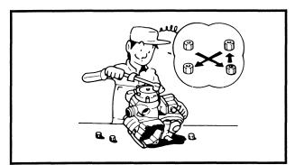
6. Be sure to keep to tightening torque specifications. When tightening bolts, nuts, and screws, start with larger-diameter pieces, and proceed from an inner-positioned one to an outer-positioned one in a criss-cross pattern.
