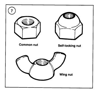
cation, but without the length dimension. The measurement across two flats of the nut indicates the wrench size required to turn the nut.
