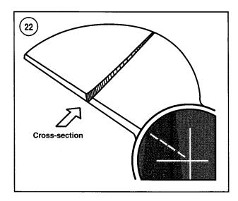
shaped cross-section (**Figure 22**). The leading edge is very thin and the blade thickness increases toward the trailing edge, where it is thickest. If a propeller such as this is run totally submerged, it is very inefficient.
