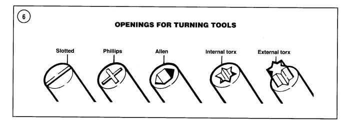
face. Figure 6 shows a number of screw heads requiring different types of turning tools.
