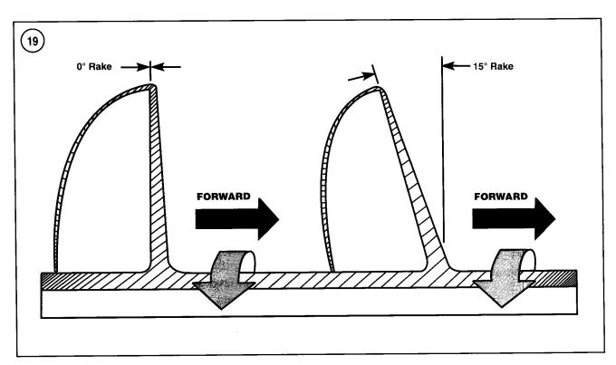
hub (**Figure 19**) has 0° rake. A blade that is angled from perpendicular (**Figure 19**) has a rake expressed by its difference from perpendicular. Most propellers have rakes ranging from 0-20°. Lighter faster boats generally perform better with propeller with a greater amount of rake. Heavier, slower boats generally perform better using a propeller with less rake.
