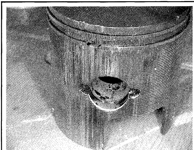
Fig. 2 This scuffed piston is an example of what can happen when the proper 2-stroke oil is not used. The outboard required a complete overhaul
