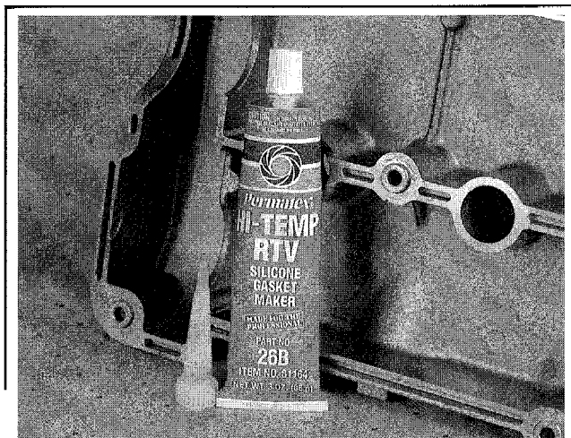
Fig. 7 On some engines, RTV is used instead of gasket material to seal components
