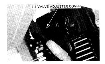
Remove the camshaft inspection hole cap from the cylinder head cover and check that timing mark on the camshaft is visible (facing up).
