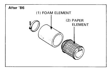
Wash the foam element in clean soapy water and squeeze out the excess water.
