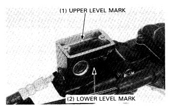
Check the front and rear brake fluid reservoir levels.
