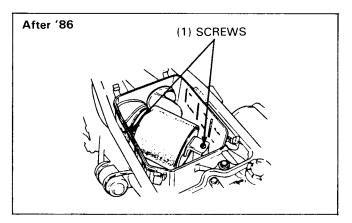
Remove the foam element from the paper element.
