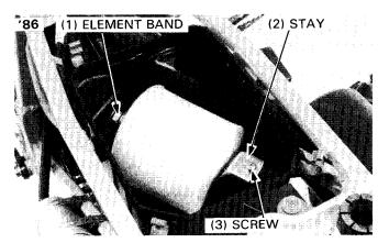
Wash the element in non-flammable or high flash point solvent, squeeze out the solvent thoroughly, and allow the element to dry.
