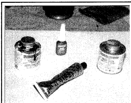
Fig. 31 Sealants are essential for preventing leaks
