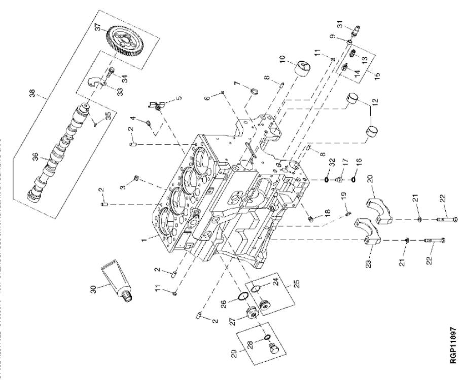
John Deere > Turf And Utility >TRACTOR >5725N - TRACTOR >5425N and 5725N Narrow Tractors (Worldwide Edition) >20 ENGINE 4045DP052-RE517022 >ST685870 - 4607 CYLINDER BLOCK FITTINGS, MAIN BEARING CAPS
