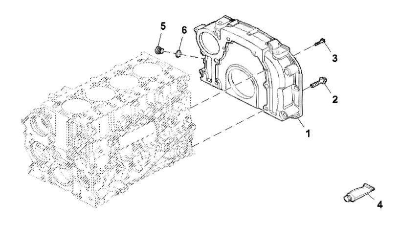
John Deere > Turf And Utility >TRACTOR >F5GFL413L - TRACTOR >5090GV Tractor (Engine F5G) FT4 (North America Edition) >20 ENGINE >ST845945 - FLYWHEEL HOUSING
