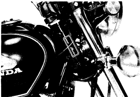
The frame serial number is stamped on the steering head right side.
